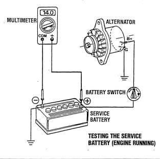
**CAUTION:** When performing tests on the alternator charging circuit do not use a high voltage tester (i.e. Megger). You can damage the alternator diodes
