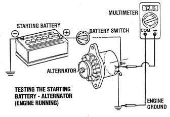
**f.** Start the engine again. Check the voltage between the alternator output and ground.
